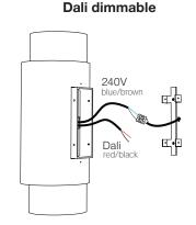
Installation options for standard dimmable version or Dali dimmable version. JSPR provides an option of purchasing a Dali dimmable version, the driver will be built-in the fixture. Use splicing connectors for direct connection.
