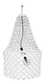
Unscrew the old bulb and replace with new LED bulb max 100W. Screw thread E27.
