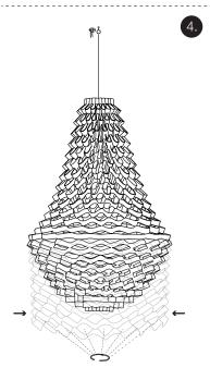
Close the bottom of the Crown with small clip-ring provided. Pull through all holes of the bottom layer.
