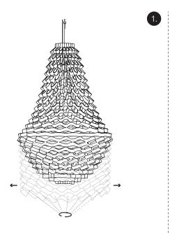
To replace the large bulb the light fixture must be opened from the bottom. Carefully locate the bottom ring and unclick to open the ring.
