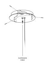
Fix cover plate to the base plate with three/four included screws. Once tightly fixed proceed to hanging the lamp by guiding the lamps suspension cable through the little nozzle located on the canopy. Tuck away any excess electricity cables into canopy.
