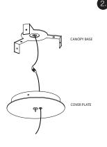
Guide the lamps electricity cable to the canopy cover plate. Connect the house electricity cable to the lamps electricity cable. Use a conection block to make a safe connection.
