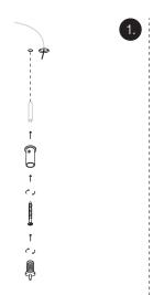
Carefully unpack the lamp and untwine the electric wire and suspension cable. Mark and drill a hole next to the house wire. Use a dowel and a hook (by client); JSPR ceiling fasteners or JSPR canopy (instructions in this manual).
