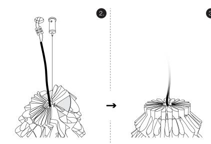
Attach the suspension cable to the hook/JSPR ceiling fastener, adjust desired cable length and tighten the cable fastener. Trim excess cable. Connect the electricity using electric connection blocks. and proceed to arrange the top plate of the lamp.
