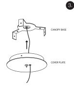
Once the electricity cables are connected attach the cover plate to the premounted canopy base.
