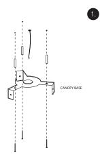
Mark holes in the ceiling based on canopy measurements. Attach canopy base plate using screws and plugs (by client, depending on ceiling material).
