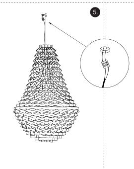
Finally connect the lamps electric wire to the house wire. Arrange all layers/flaps that have turned inside out to match drawing.
