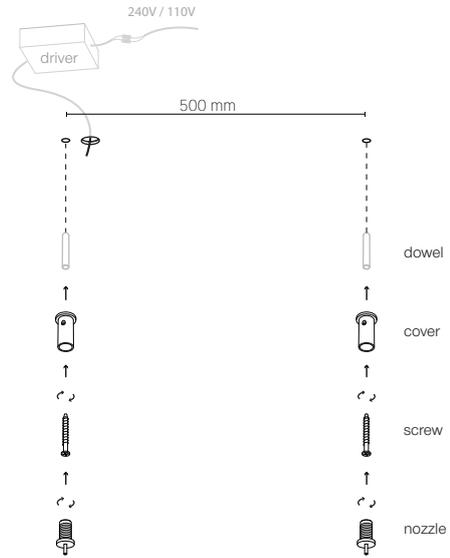
Guide the suspension cables through the fasteners. Keep adjusting the suspension cables to reach desired height and level. Detailed description of the use of JSPR ceiling fasteners is enclosed in this document.
