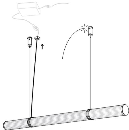
Tuck away any loose electric cable and trim the suspension cable once the desired level and length is reached.
