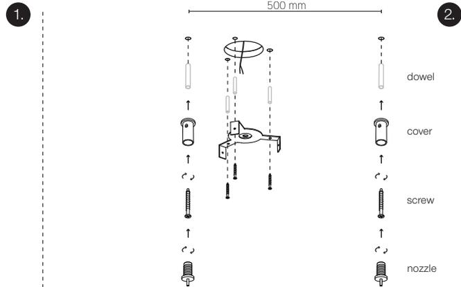
Mark and drill holes around the house electricity wire based on the ceiling bracket and additional 2x holes to hold the suspension cables.
