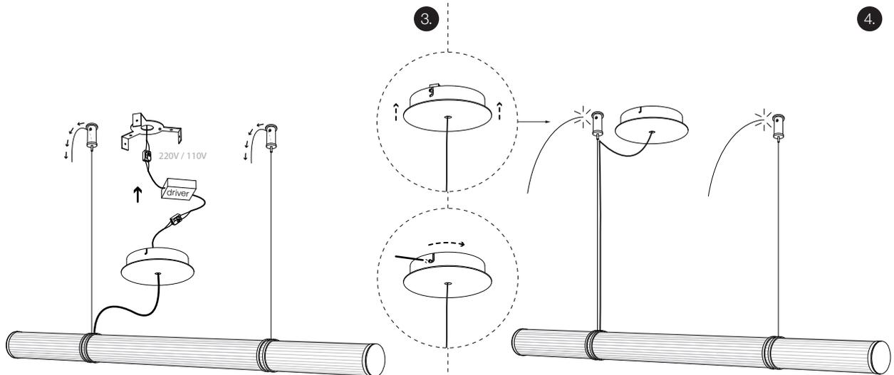
Guide both suspension cables through the premounted ceiling fasteners. Guide the low voltage electricity cable through the canopy base and connect fixtures electric cable to the driver cables minding the markings + to +; - to - with a connector clip (provided).
