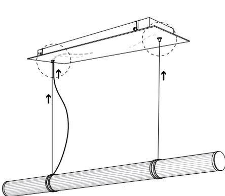
Extended or shorten suspension cables pushing or pulling into the canopy to level the fixture. Tuck any excess electricity cable in the canopy.
