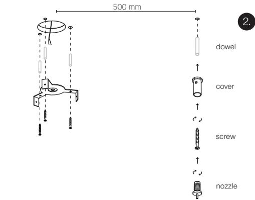
Mark and drill holes around the house electricity wire based on the ceiling bracket.
