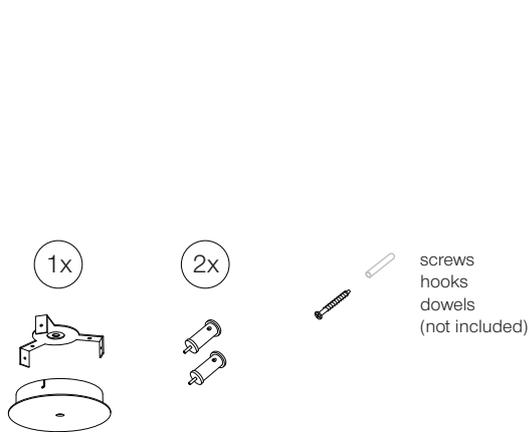
Carefully unpack the light fixture. Set includes Canopy and **2x** JSPR ceiling fastener. Uncoil the suspension cables and electric cable. Unscrew the nozzle parts of the ceiling fasteners from the cover parts. Split the canopy from the ceiling plate.
