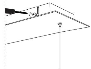
Tighten screws to fix position.
