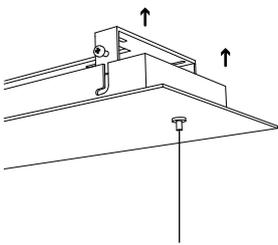
Align the canopy cover to the ceiling bracket screws and push the cover over the ceiling bracket.
