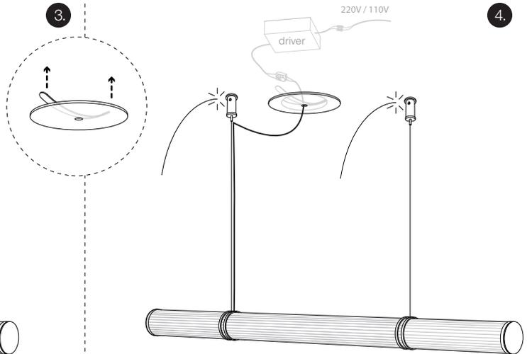
Gently bend the canopy flaps upwards and release above the dropped ceiling. This will fix the canopy plate and cover up the drop ceiling opening.
