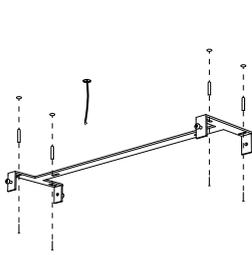
Carefully unpack the light fixture. Locate the ceiling bracket. Mark and drill holes near the house electricity wire based on ceiling bracket.
