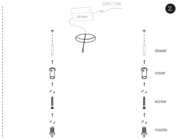
Mark and drill holes into solid structure that safely holds the fixture.
