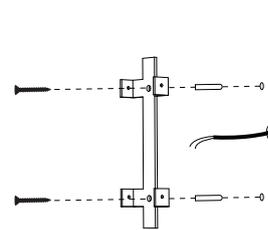
Mark and drill holes in the wall near the house electricity cable. Use screws and dowels to fasten the wall bracket.
