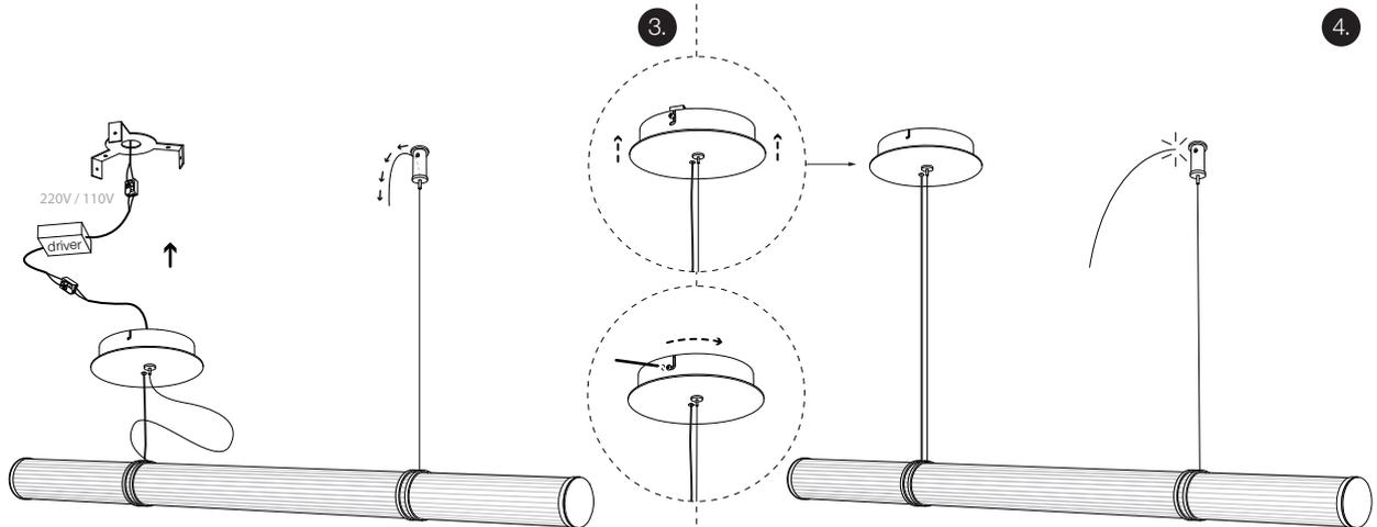
Guide the electricity cable and suspension through the canopy base. Fix both suspension cables to the ceiling. Level the light fixture and proceed to connect the LED driver following instructions on the driver. Connect the driver to the light fixture minding the markings + to +; - to - with a connector clip (provided).
