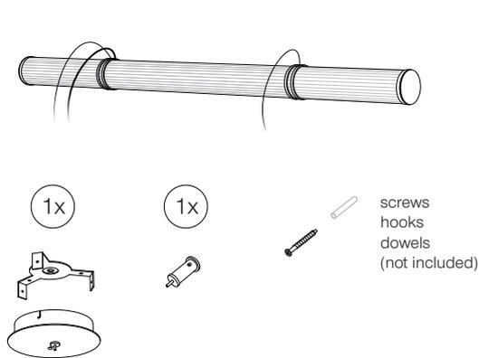
Carefully unpack the light fixture. Set includes Canopy and **1x** JSPR ceiling fastener. Uncoil the suspension cables and electric cable. Unscrew the nozzle part of the ceiling fastener from the cover parts. Split the canopy from the ceiling plate.
