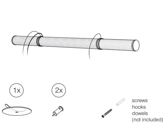
Carefully unpack the light fixture. Set includes flat canopy and **2x** JSPR ceiling fasteners. Uncoil the suspension cables and electric cable. Unscrew the nozzle parts of the ceiling fasteners from the cover parts.
