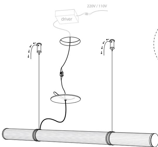
Guide both suspension cables through the premounted ceiling fasteners. Guide the low voltage electricity cable through the flat canopy and connect fixtures electric cable to the driver cables minding the markings + to +; - to - with a connector clip (provided).
