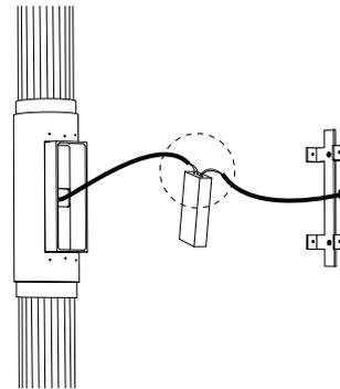
Installation option with or without dimmer unit. JSPR provides an option of purchasing dimmers for the Union series that fit within the wall box. Use splicing connectors for direct connection. In the case of using a dimmer module follow the included instructions of the dimmer.
