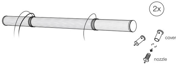
Carefully unpack the light fixture. For this setup **Pillar** suspended lights require **2x JSPR ceiling fasteners** (included). Uncoil the suspension cables and electric cable. Unscrew the nozzle parts of the ceiling fasteners from the covers.
