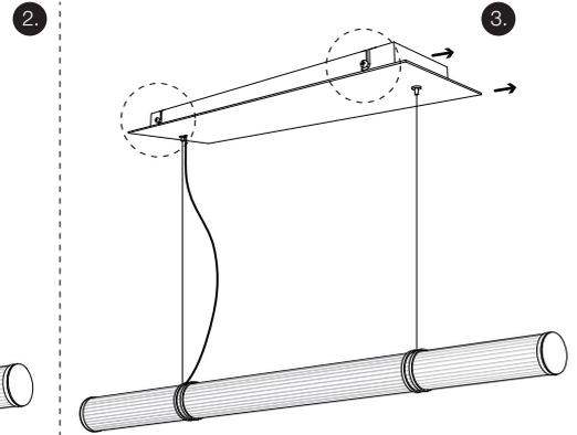
Align the plate against the ceiling bracket screws and pull sideways to hook it on. Use screwdriver to tighten the bracket screws and fix the canopy cover to the pre-installed ceiling bracket.
