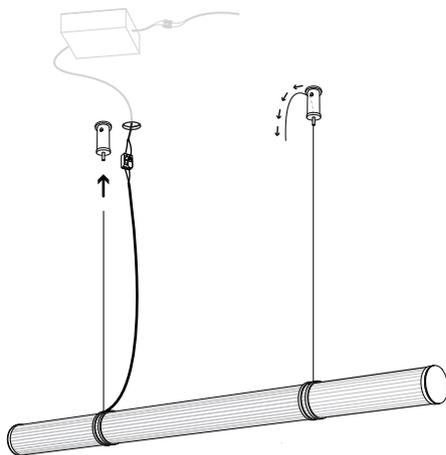
Mark and drill holes near the electricity cable from the built-in driver. Suspension cable distance between all Pillar suspended models is 50cm.
