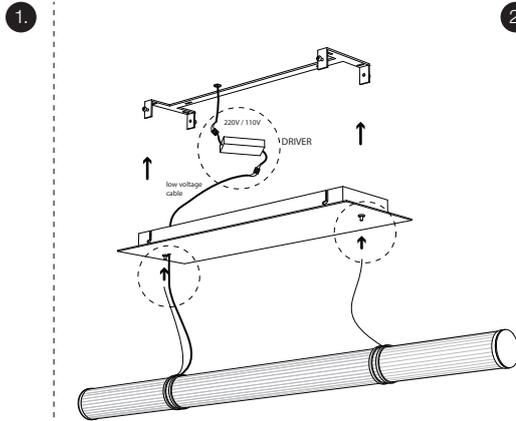
Shorten suspension cables and electricity cable leaving extra length for alignment. Guide the suspension cables through the fasteners on canopy (manual for how these are adjusted is enclosed in this document). Pull-through fixtures electricity cable through the cover plate and connect the necessary driver.
