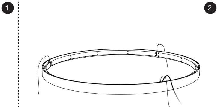
Carefully unwrap the fixture on a soft clean surface. Locate all cable fasteners on the top of the lamp. Uncoil the provided suspension cables and electric cable.
