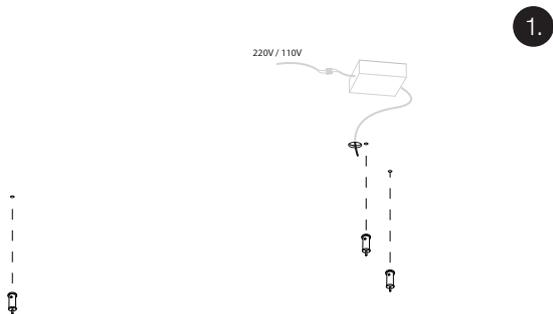
Mark and drill holes in the ceiling based on lamp measurements. Attach JSPR suspension cable fasteners positioning one near the built - in ceiling.
