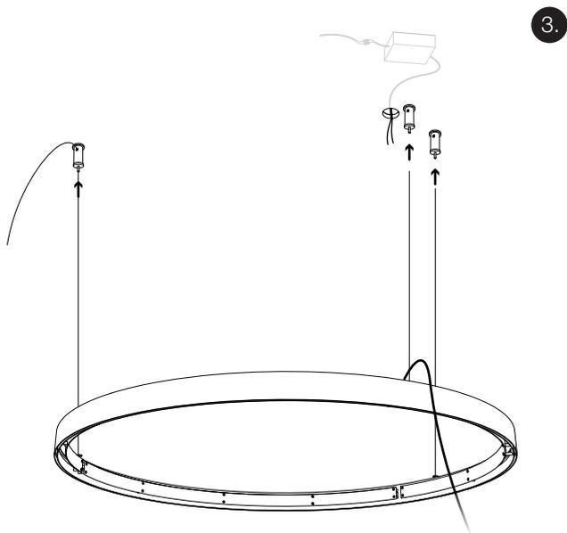
Guide the lamps suspension cables through the pre-mounted ceiling fasteners until desired length is achieved.
