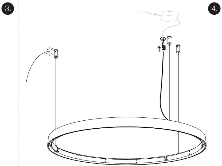
Shorten the electric wire and connect it to the transformer wires (check the markings “+” and “ - ” provided on the parts), use provided splicing connectors. Tuck away any excess wires and trim suspension cables if necessary.
