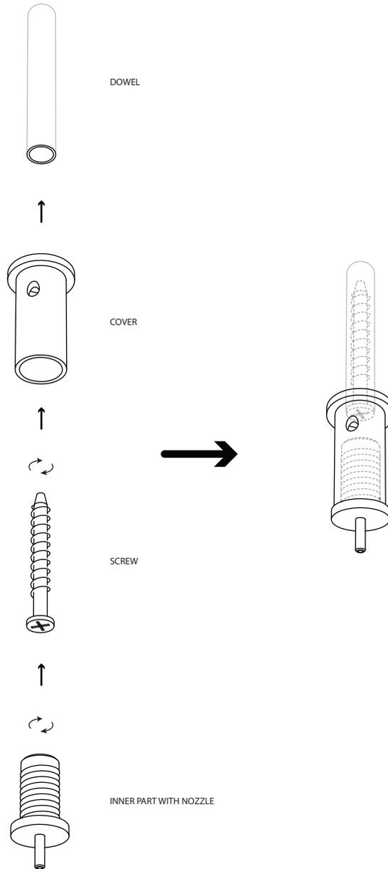
Drill hole in the desired location in the ceiling, place a dowel in the hole (dowel and screw by client). Fasten the cover of the cable fastener with a screw by guiding it through the cover into the dowel. Once the cover is fastened screw in the inner part of the cable fastener.
