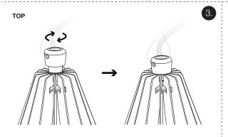
Once all panels are inserted fix them in place by screwing the top cap.
