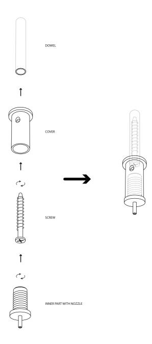
Drill hole in the desired location in the ceiling, place a dowel in the hole (dovel and screw by client). Fasten the cover of the cable fastener with a screw by guiding it through the cover into the dowel. Once the cover is fastened screw in the inner part of the cable fastener.
