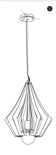
Mark and drill holes in the ceiling near the house electricity wire, based on the canopy size. Attach canopy base plate using screws and dowels (by client).
