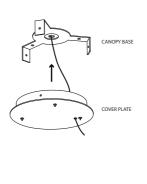
ASSEMBLY WITHOUT DRIVER Pull through cover plate the house electricity cable or connect the lamps electric cable (through cover plate) to the house electricity wire.
