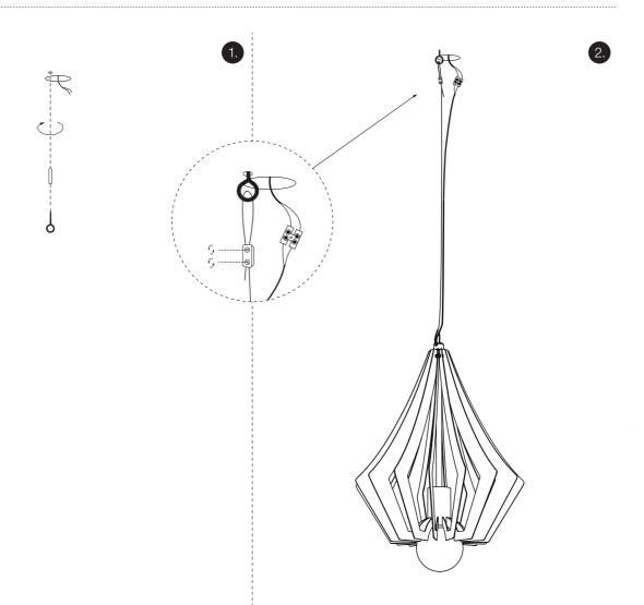
Near the house electric wire drill a hole in the ceiling for a suspension hook (provided by client). Use a dowel to secure the hook in the ceiling.
