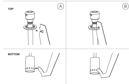
Take a panel and allign it to an opening on the top of the core of the lamp and on the bottom where the bulb will later on come.
