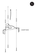
Mark holes in the ceiling based on canopy measurements. Attach canopy base plate using screws and plugs (by client).
