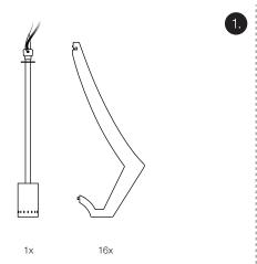
Carefully unpack the light fixture. The box contains 1x core with pre assembled wiring and 16x lamp shade panels.
