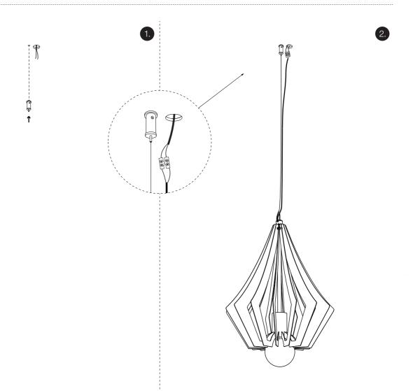
Mark and drill a hole in the ceiling next to the house electricity cable. Attach JSPR suspension cable fastener (sold separately) using a screw and dowel (by client).
