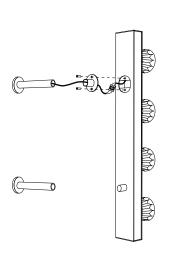
Connect the house electricity wire to the lamp. Tuck away any excess wire in the fixture and attach the cap back to the lamp.
