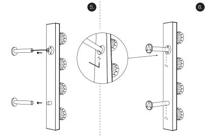
Slide the light fixture on the brackets by carefully aligning the top and bottom bracket to the lamp.
