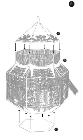
After assembling the top (A) and body (B) connect them using the same bolts and nuts provided and continue by adding the base hexagon (C).
