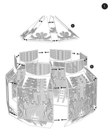
Assemble the top/roof (A) part of the cage and the body (B) of the cage using the bolts and nuts provided. Both parts each consist of six modules.
