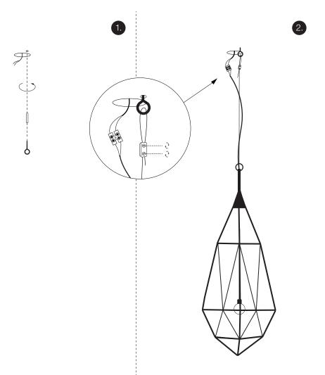
Near the house electric wire drill a hole in the ceiling for the suspension hook (provided by client). Use a dowel to secure the hook in the ceiling.
