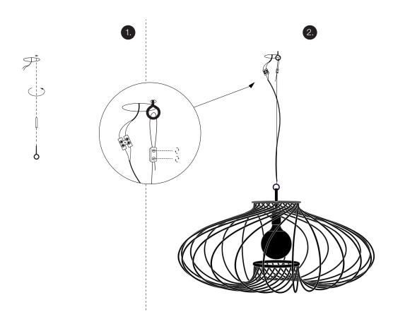
Near the house electric wire drill a hole in the ceiling for a suspension hook (provided by client). Use a dowel to secure the hook in the ceiling.
