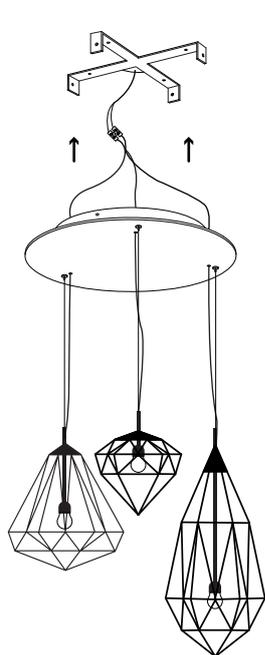
4. Connect each lamps electricity cable to the house electricity cable and tuck all excess cables inside the cover plate before attaching the cover plate to the base plate.
