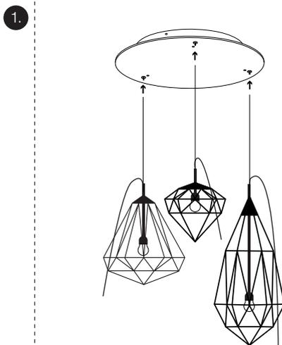
2. Carefully unwrap the Diamond lights and guide the suspension cables through the cable fasteners located on the cover plate.
