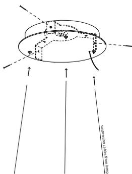
Fix cover plate to the base plate with three included screws. Once tightly fixed proceed to hanging the lamp by guiding the lamps suspension cables through the little nozzles.
