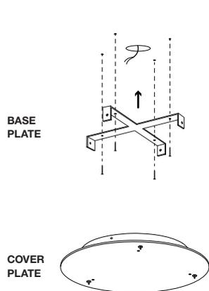
1. Mark and drill holes in the ceiling based on the base plate size. Carefully unwrap and attach the base plate to the ceiling using dowels and screws (by client).
