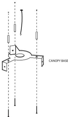
Mark holes in the ceiling based on canopy measurements. Attach canopy base plate using screws and plugs (by client).
