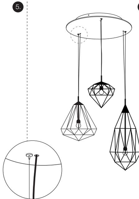
6. Adjust the desired length of each pendant. Detailed instructions how to use integrated cable fasteners included in this manual.
