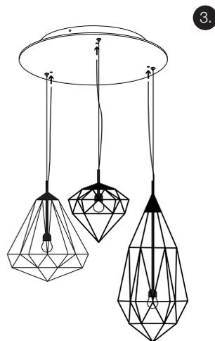
3. Pull through each Diamonds electric cable through the cover plate.
